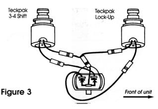
The Lock-up solenoid is located nearest the front of the transmission. The wire located closest to the front of the transmission is the 3-4 ground. This is the solenoid located to the rear. Make wire connections as shown in **Figures 2 and 3**.
