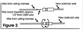
4. Strip back lead wires cut from the old solenoid and original solenoid harness approximately 1/2" and twist braided wire to form a tight strand. Loosen the Posi-Lock<sup>™</sup> Connectors. Insert the bare wire into the connector until it bottoms out. Tighten the connector. Repeat this procedure for all of the connections. See **Figure 2**.
