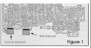
2. After the valve body has been removed, the separator plate must be removed. Now remove the retainer clips that keep the solenoid in place. Remove the Lock-up solenoid. Cut the wires as close as possible to the Lock-up solenoid.
