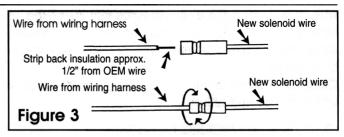
5. Strip back lead wires cut from the old solenoid and original solenoid harness approximately 1/2" and twist braided wire to form a tight strand. Loosen the Posi-Lock™ Connectors. Insert the bare wire into the connector until it bottoms out. Tighten the connector. Repeat this procedure for all of the connections (Figure 3).
