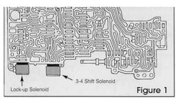
2. After the valve body has been removed, the separator plate must be removed. Now remove the retainer clip that keeps the solenoid in place. Cut the wires as close as possible to the Shift solenoid.
