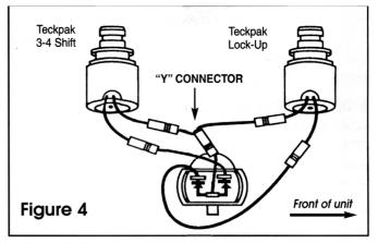
the positive center wire goes to both solenoids. The wire located to the rear of the transmission is the lock-up ground. The lock-up solenoid is located nearest the front of the transmission. The wire located closest to the front of the transmission is the 3-4 ground. This is the solenoid located to the rear. Make wire connections as shown in **Figures 3 and 4**.
