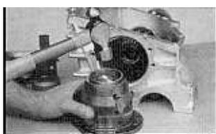
Install the new carrier bearing race. Do not use the oil splash shield when using Teckpak's Axle Stabilizers.
